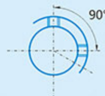
变更止动螺丝角度用KC90表示 Kc90 shows alteration of stop screw angle.
