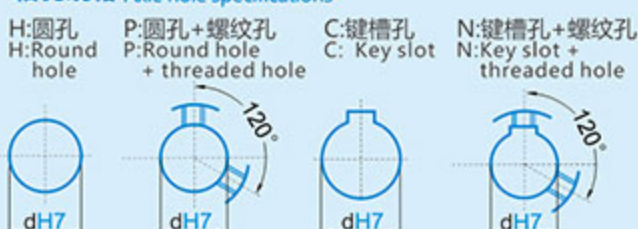
轴孔规格 Axle hole specifications
