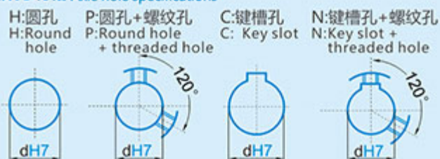
轴孔规格 Axle hole specifications
